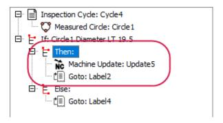
**Else** (if the diameter is not less than 19.5 mm), the process should proceed to Label 4, which is located in Operation 8.
