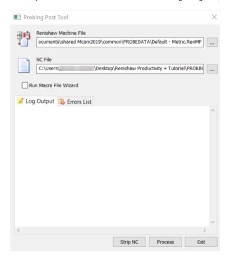
In order to successfully create probing output, you must have a post processor with probing enabled and a .RenMF customized for your specific machine. Select the .RenMF after you have initiated the post from the Probing Post Tool dialog box, or when you configure your probe operation from the Probe Configuration dialog box.
