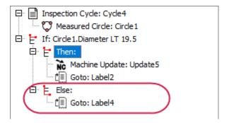
Note: Open the parameters for Operations 5 and 8 to view Label2 and Label4.
