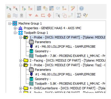
To create a probe operation, select **Probe** from the **Mill Toolpaths** or **Router Toolpaths** contextual tab.
