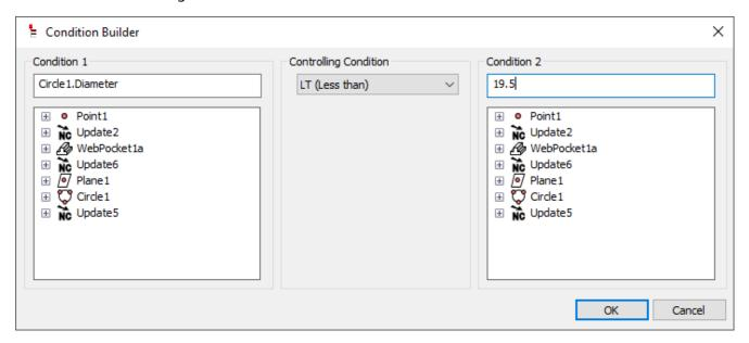
In the **Condition Builder** dialog box, a **Controlling Condition** defines the relationship between any two of the following:
